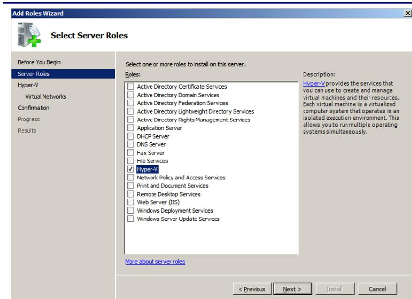
**Figure 6. Installing the Hyper-V role in Windows Server 2008 R2.**
