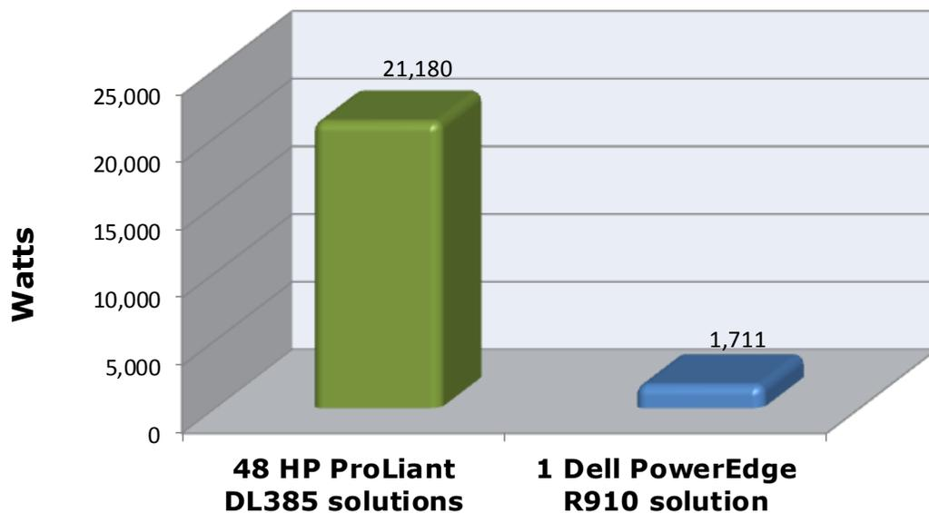
**Figure 13. Estimated power usage under typical load for the single Dell PowerEdge R910 solution and 48 HP ProLiant DL385 solutions. Typical power is the average of idle power and power under load. Lower results are better.**
