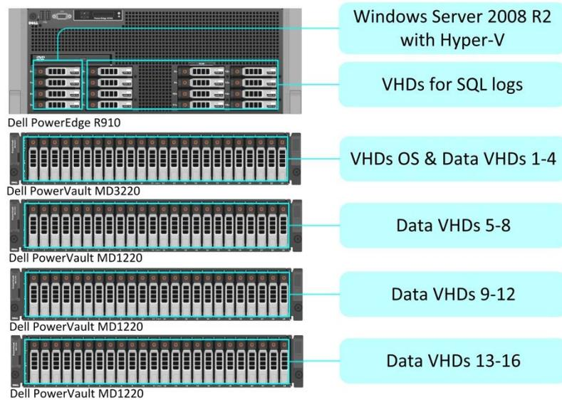
**Figure 2. Disk layout for our virtualized SQL Server 2008 R2 testing.**
