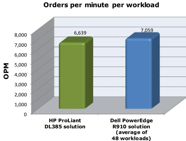
**Figure 3. Average OPM of 48 database workloads on the Dell PowerEdge R910 solution versus a single database workload on the HP ProLiant DL385 solution. Greater OPM is better.**
