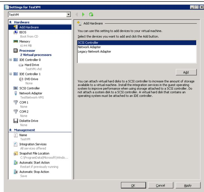
**Figure 7. Virtual Machine configuration in Hyper-V.**
