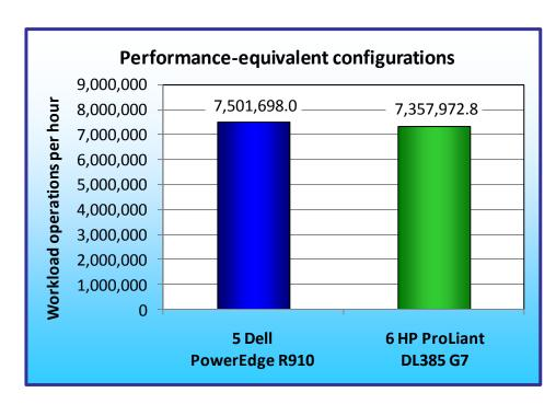
Figure 3: Performance-equivalent configurations based on representative SAP ERP workload. Higher numbers are better.
