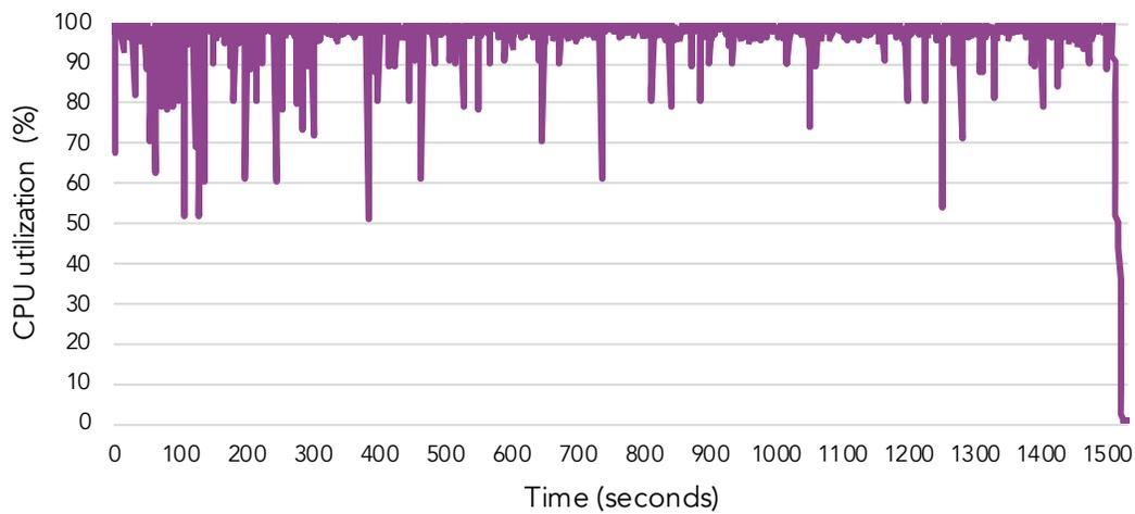
Figure 2: Graph of the HPE ProLiant DL380 Gen10 server's CPU utilization for the duration of the machine learning preparation test. Source: Principled Technologies.
