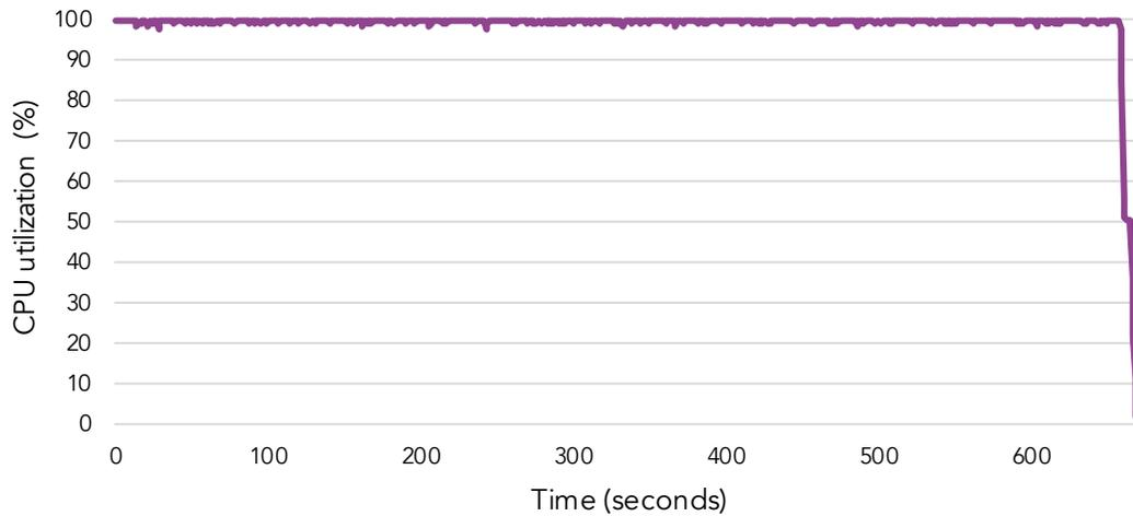
Figure 1: Graph of the Dell EMC PowerEdge R7525 server's CPU utilization for the duration of the machine learning preparation test. Source: Principled Technologies.
