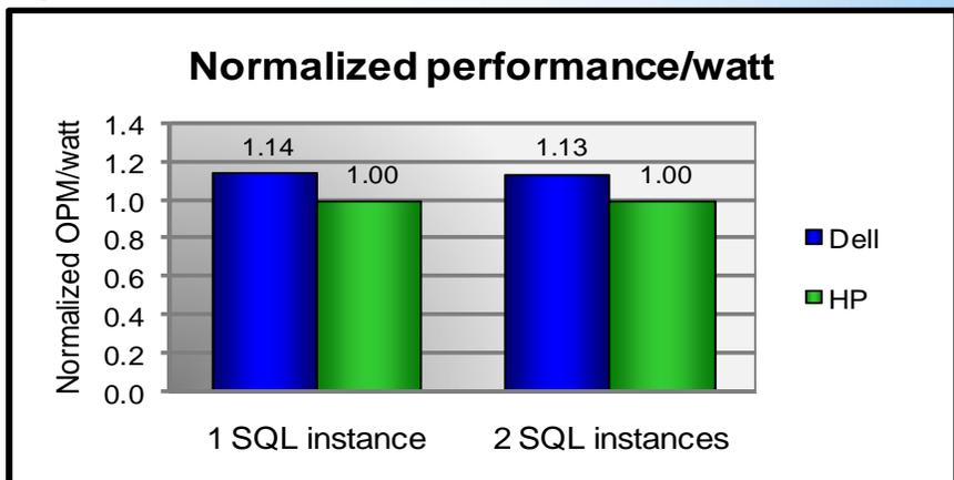
Figure 3: One- and two-database-instance normalized performance/watt results. Higher numbers are better.
