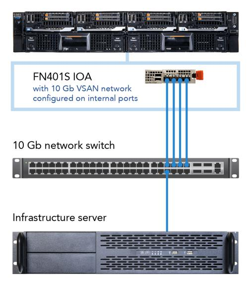
Figure 8: Our testbed for the Dell PowerEdge FX2 solution.
