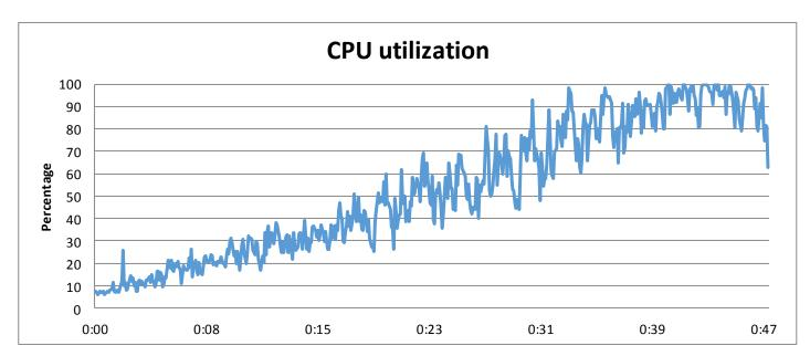
Figure 10: CPU utilization throughout our test period for the legacy Cisco server using a traditional SAN with one B200 M2 blade.
