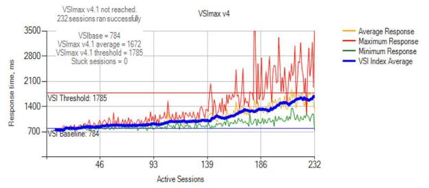
Figure 8: The legacy Cisco server using a traditional SAN with four B200 M2 blades ran 232 sessions and did not reach VSImax; Adding additional sessions caused the server to reach VSImax due to CPU saturation and unacceptable end-user response times.
