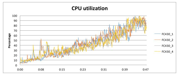
Figure 11: CPU utilization throughout our test period for the Dell PowerEdge FX2 using VMware Virtual SAN with four FC430 sleds.
