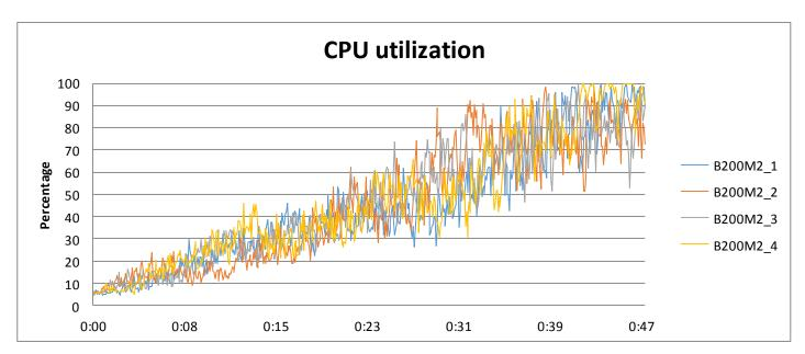
Figure 12: CPU utilization throughout our test period for the legacy Cisco server using a traditional SAN with four B200 M2 blades.
