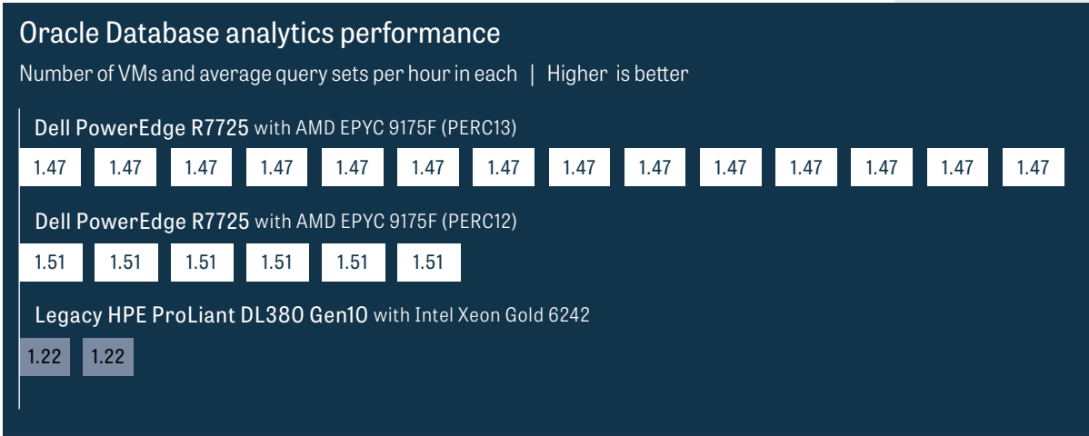
Figure 2. Oracle Database analytics performance, in number of VMs and average query sets per hour in each VM, for the solutions. Source: PT.
