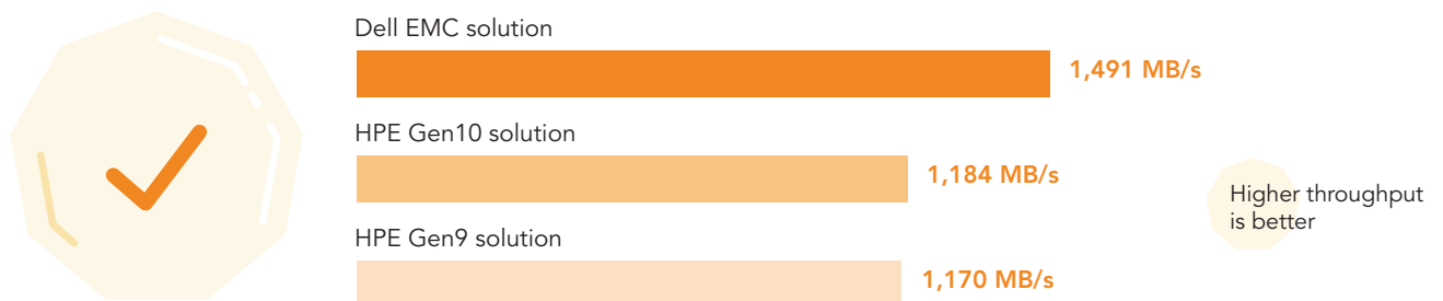
Figure 2: Disk-read throughput (in megabytes per second) achieved by each solution while running a TPC-H-like data analytics workload. Higher throughput is better. The Dell EMC solution comprised three Dell EMC PowerEdge servers and a PowerStore 5000T storage array. The HPE Gen9 solution used three HPE ProLiant DL380 Gen9 servers, while the HPE Gen10 solution had three HPE ProLiant DL380 Gen10 servers. Both HPE solutions used a 3PAR StoreServ 8450 storage array. Source: Principled Technologies
