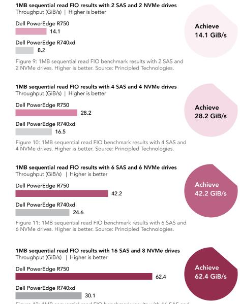
Figure 12: 1MB sequential read FIO benchmark results with 16 SAS and 8 NVMe drives. Higher is better. Source: Principled Technologies.
