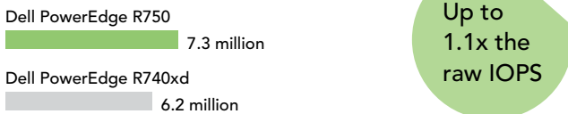
Figure 2: Random write FIO benchmark results on 24 NVMe drives with 56 cores for the PowerEdge R750 and 36 cores for the PowerEdge R740xd. Higher is better. Source: Principled Technologies.
