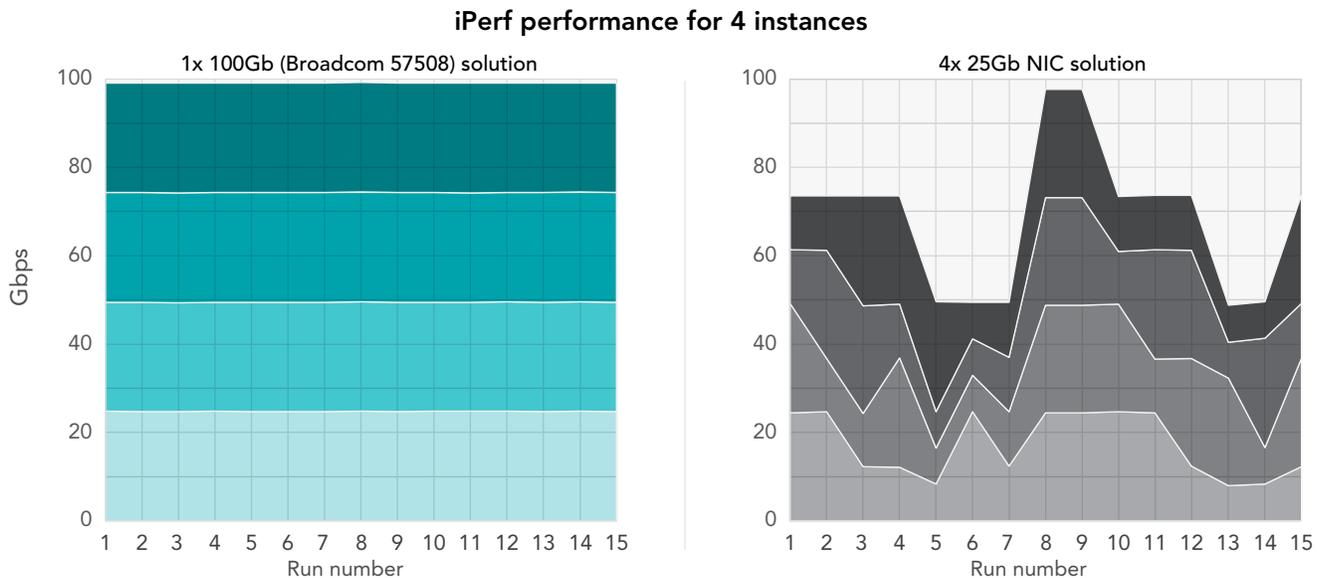
Figure 2: iPerf results, in Gbps, for four TCP streams. Higher numbers and more consistency is better. Source: Principled Technologies.
