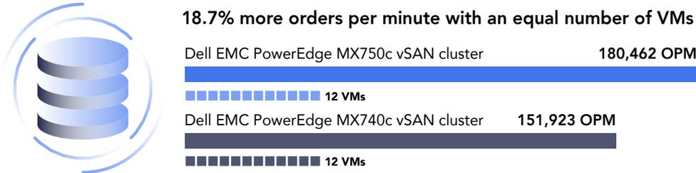
Figure 1: Total OPM the 2 clusters achieved with 4 VMs/node. Higher is better. Source: Principled Technologies.
