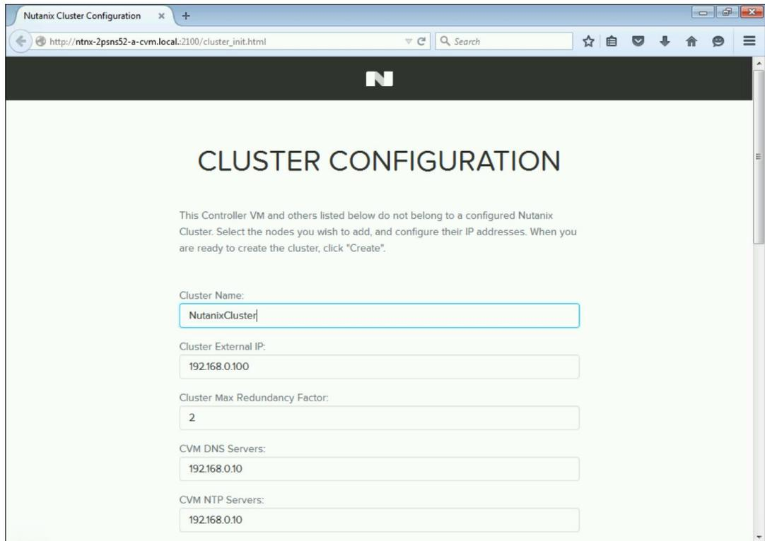
Figure 5: Providing a cluster name, external IP, CVM DNS server, and CVM NTP server.
