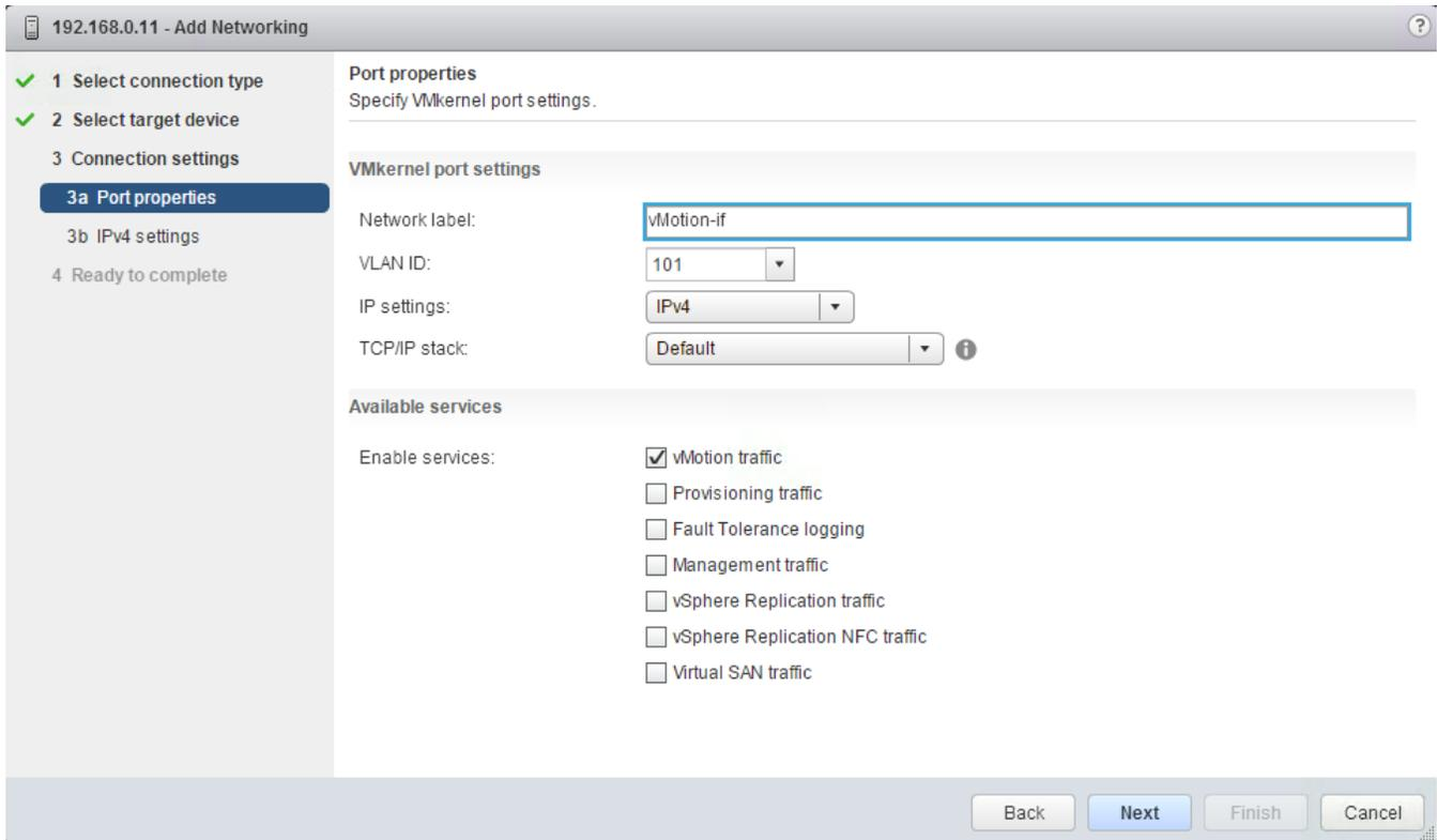
Figure 19: Enabling vMotion traffic and setting the appropriate VLAN ID on a new VMkernel port.
