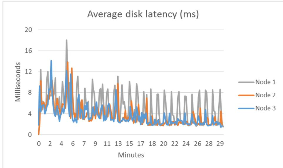
Figure 25: Average disk latency for each Dell XC630 host's disks.
