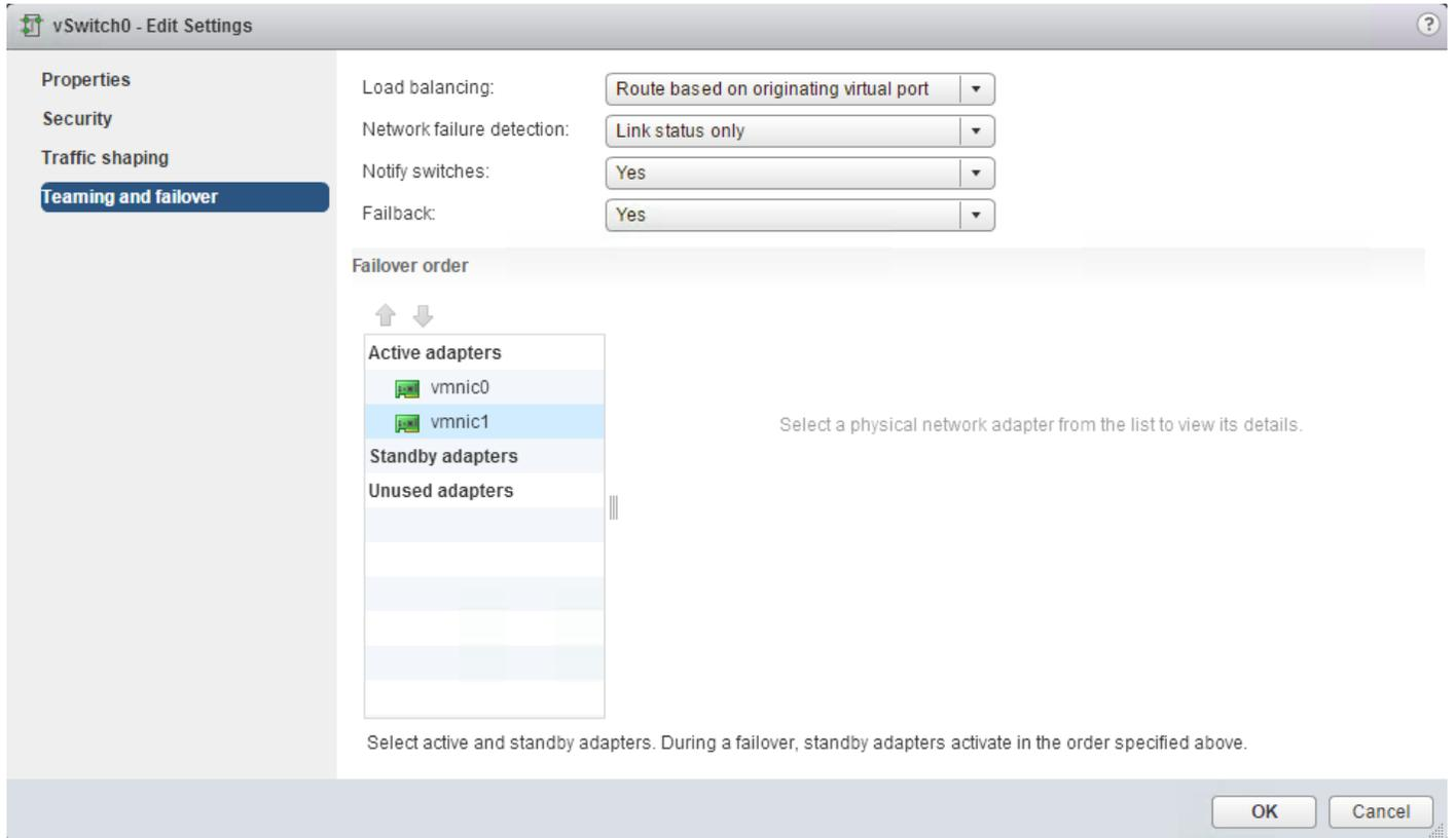
Figure 21: Setting both vmnic adapters to Active in the vSwitch0 NIC team in the vSphere Web Client.
