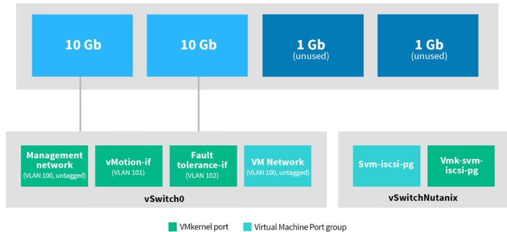
**Figure 4: The structure of each XC630 host's NIC team, formed from the two 10 Gbps ports, and their virtual switches and VMkernel ports and port groups. Note that the 1 Gbps ports are unused.**
