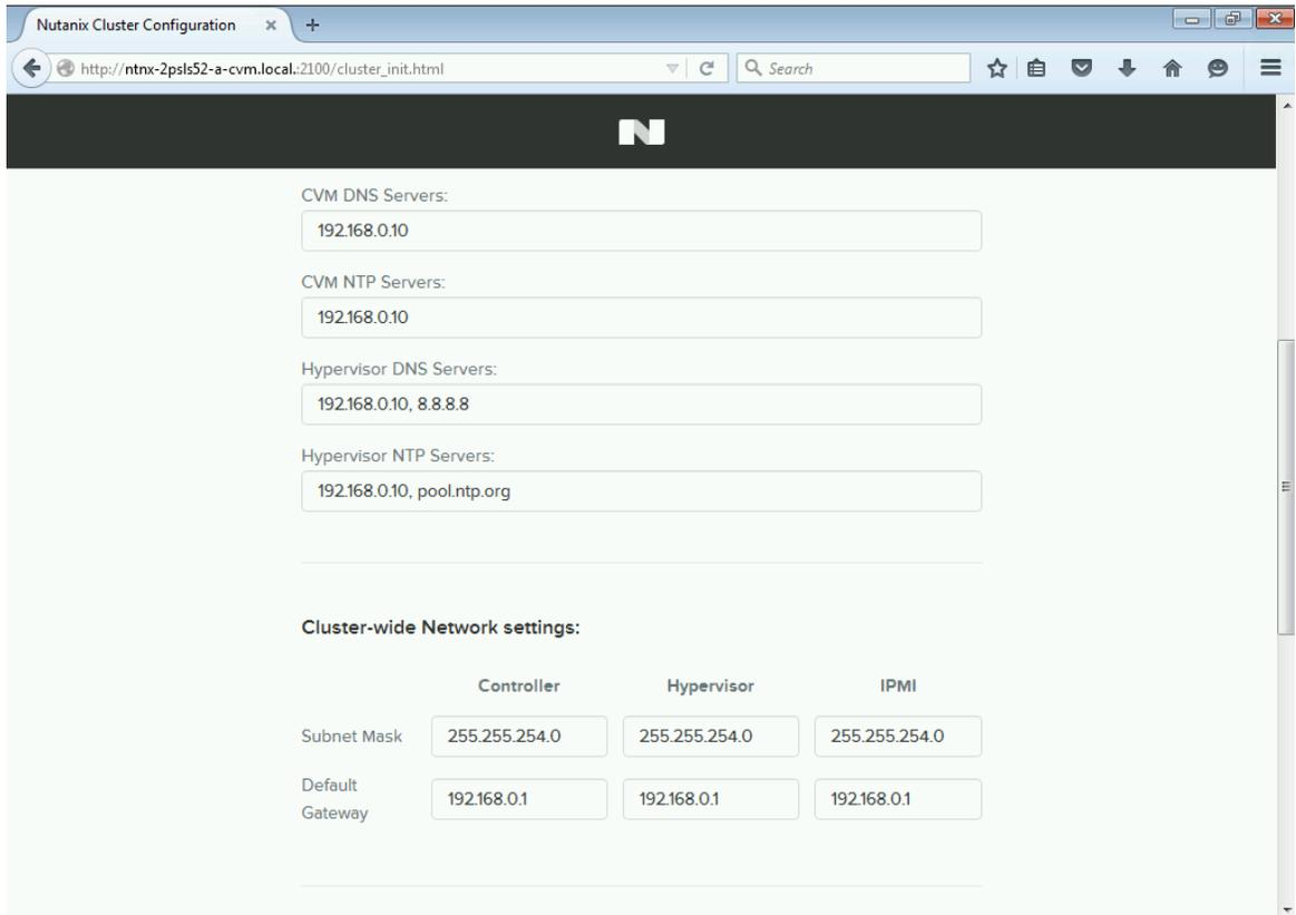
**Figure 6: Providing the appropriate subnet masks and default gateways in the Cluster-wide Network settings.**
