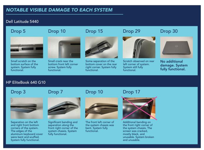
Figure 2: Images of damage to the two systems during testing.
