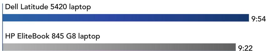
Figure 1: MobileMark 2018 overall battery life results. Time (hh:mm). More time is better.
