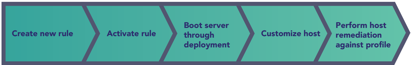
Figure 5: High-level steps necessary to deploy a host using VMware vSphere Auto Deploy. Source: Principled Technologies.
