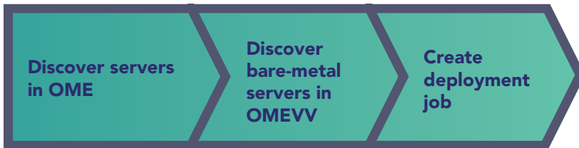
Figure 4: High-level steps necessary to deploy a host using Dell OMEV. Source: Principled Technologies.
