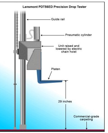
Figure 9: Our physical data protection test setup.
