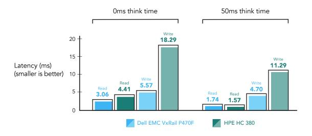
The Dell EMC VxRail solution offered up to 69 percent faster response times than the HPE solution (see chart above). In both the 0ms and 50ms think time test scenarios, the Dell EMC VxRail P470F achieved comparable or lower read and write latencies. Users expect an immediate response from their databases—and technology in general—and those fractions of seconds can pile up to make a big difference in user experience and productivity.
