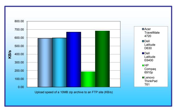
Figure 4: Upload speeds in KB/s for the five test systems. Higher numbers are better.
