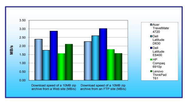
Figure 3: Download speeds in MB/s for the five test systems. Higher numbers are better.
