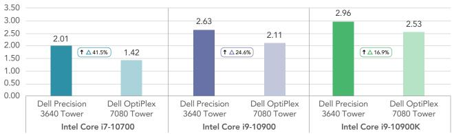
Figure 3: SPECworkstation 3 Product Development workload scores for the test systems. Higher is better. Source: Principled Technologies.
