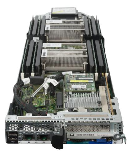
Figure 1: 1U server node of the Dell PowerEdge C6220 with the LSI MegaRAID SAS 9265-8i storage controller.
