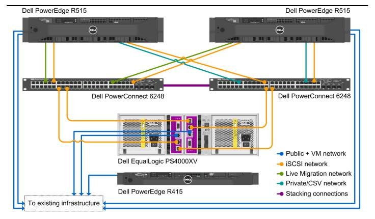
Figure 3: Networking cabling for our Dell 3-2-1 Reference Configuration.
