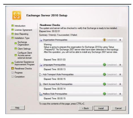
Figure 12: Readiness Checks status and install screen.
