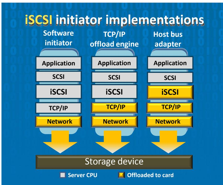
Figure 5: Three types of iSCSI initiator implementations.
