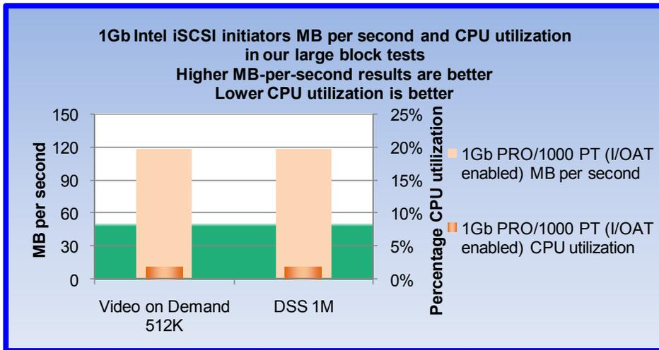
Figure 8 shows our large block test results: average CPU usage and MB-per-second output during large block tests on the 1Gb Intel PRO/1000 PT Server Adapter with I/OAT enabled. Each result is the average of the CPU utilization results that Iometer reported during individual large block tests. Higher MB-per-second and lower CPU utilization results are better.
