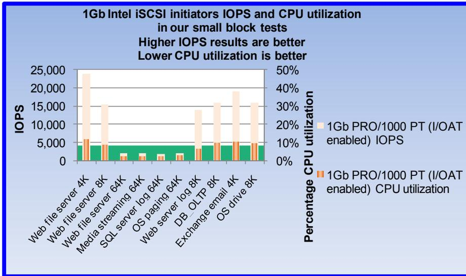
Figure 10: IOPS and CPU results for the 1Gb Intel PRO/1000 PT Server Adapter with I/OAT enabled and disabled in our small block tests. The solid green background represents 8 percent CPU usage.
