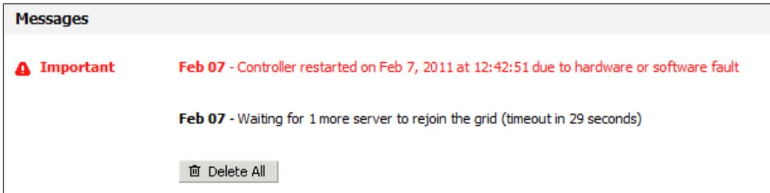
Figure 3: Hardware fault message on the CA AppLogic dashboard.
