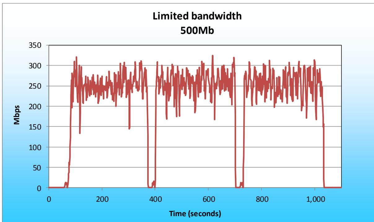
Figure 5: Network bandwidth with a limitation of 500 Mb.
