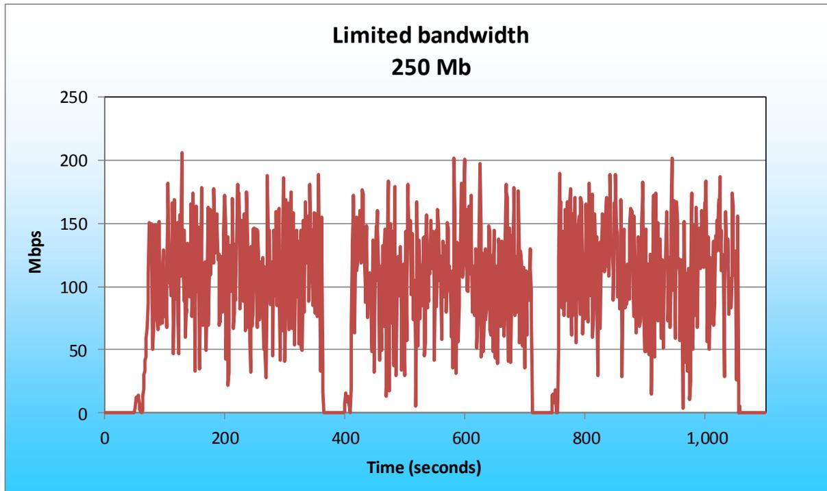
Figure 4: Network bandwidth with a limitation of 250 Mb.
