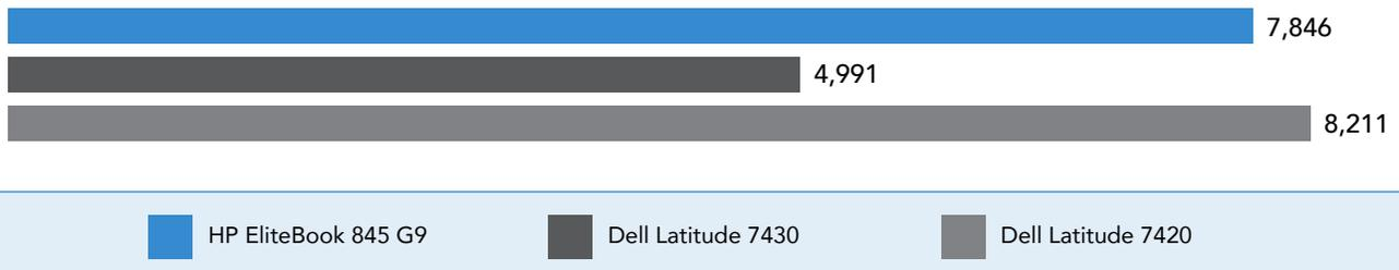
Figure 10: Productivity ratings as reported by PCMark 10 for the three systems we tested while unplugged. Higher is better. Source: Principled Technologies.
