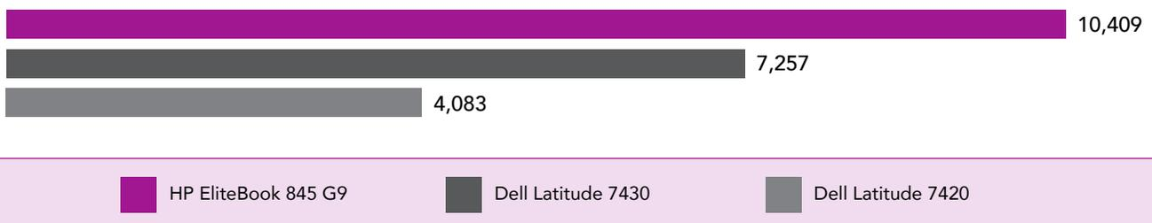
Figure 15: Sustained average Cinebench R23 multi-core scores for the three devices we tested. Higher scores are better. Source: Principled Technologies.
