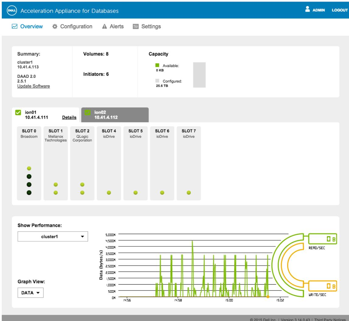
**Figure 2:** A sample of the DAAD 2.0 web GUI overview tab, with at-a-glance volume information, port connectivity, and live read/write performance monitoring.
