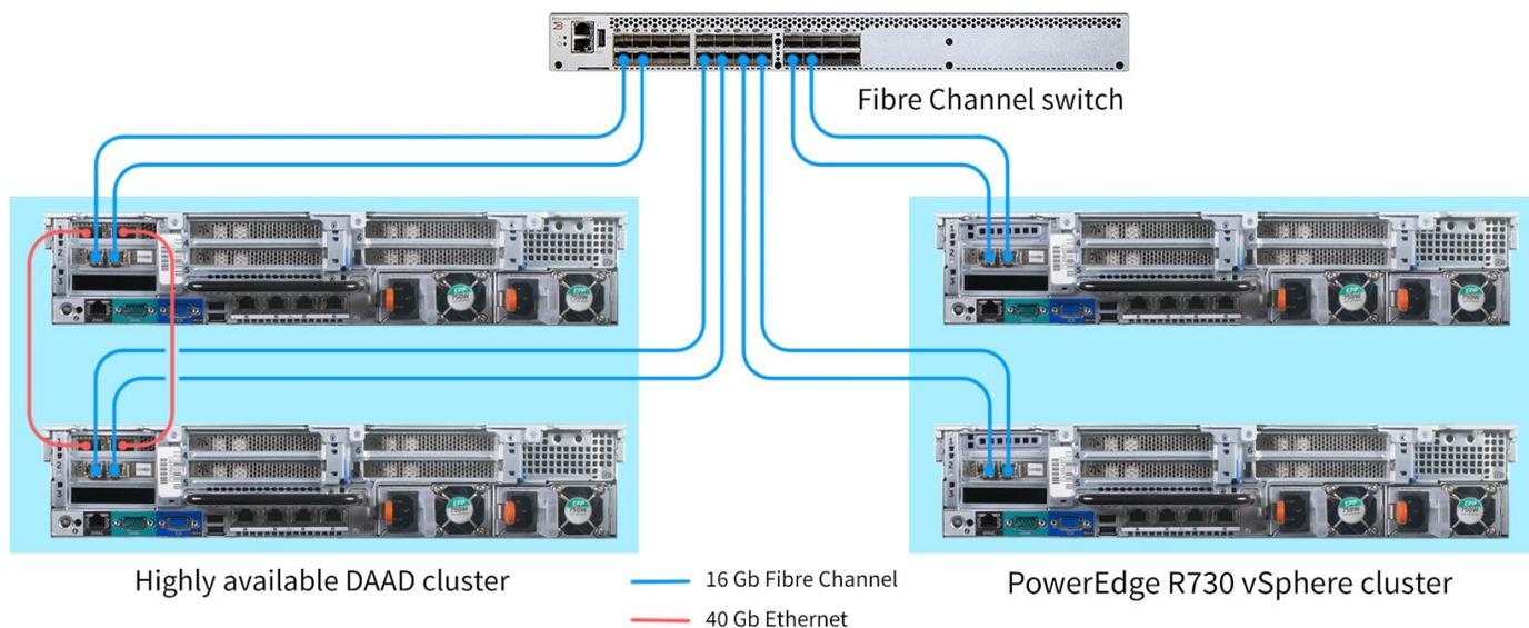
Figure 9: The back of the DAAD 2.0 connected to the other solution components.
