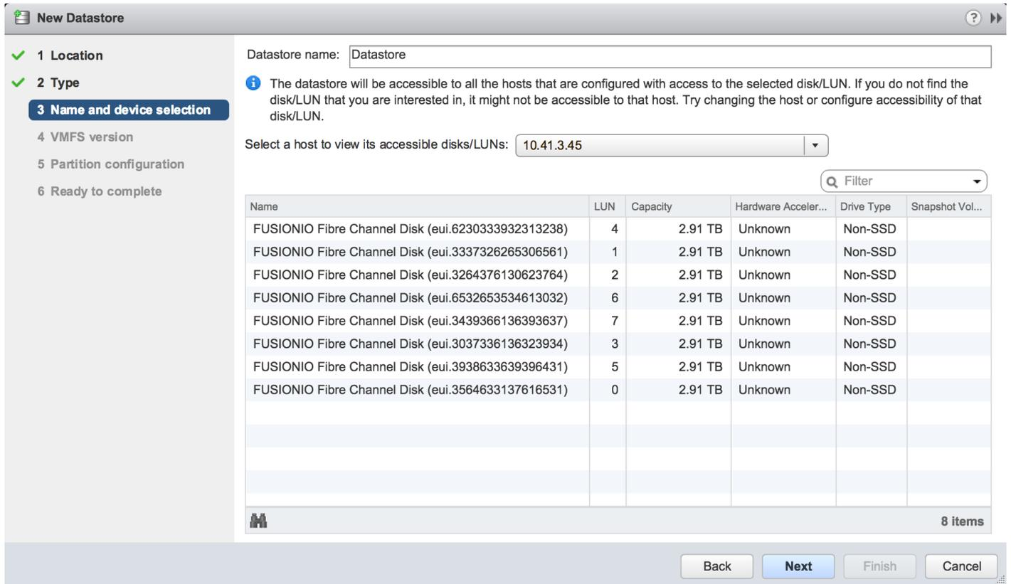
Figure 11: Discovering and adding the DAAD 2.0's LUNs to the vSphere cluster as datastores.
