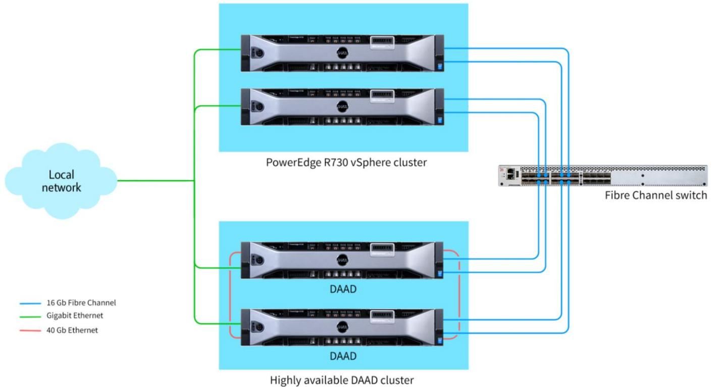
**Figure 7: Our virtualized SQL Server 2014 environment, with storage powered by DAAD 2.0, for this reference architecture.**
