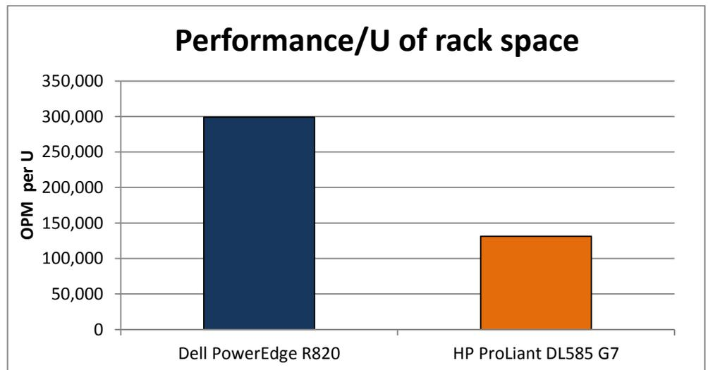
A standard 42U rack could hold 21 2U Dell PowerEdge R820 servers, for an estimated 12,562,011 OPM per rack, or hold 10 4U HP ProLiant DL585 G7 servers for an estimated 5,251,310 OPM per rack (extrapolating the performance data from our testing). That is an estimated performance increase of 139.2 percent per rack using Dell PowerEdge R820 servers.
