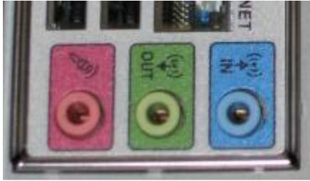
**Figure 3: Audio interface for AMD-based HP m1050e.**
