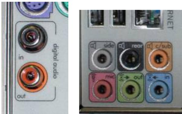
**Figure 2: Audio interfaces for the Intel-based HP m1050y.**
