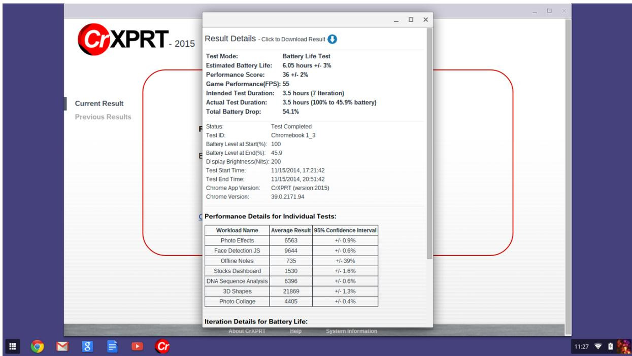
Figure 8: Detailed results for a battery life test.
