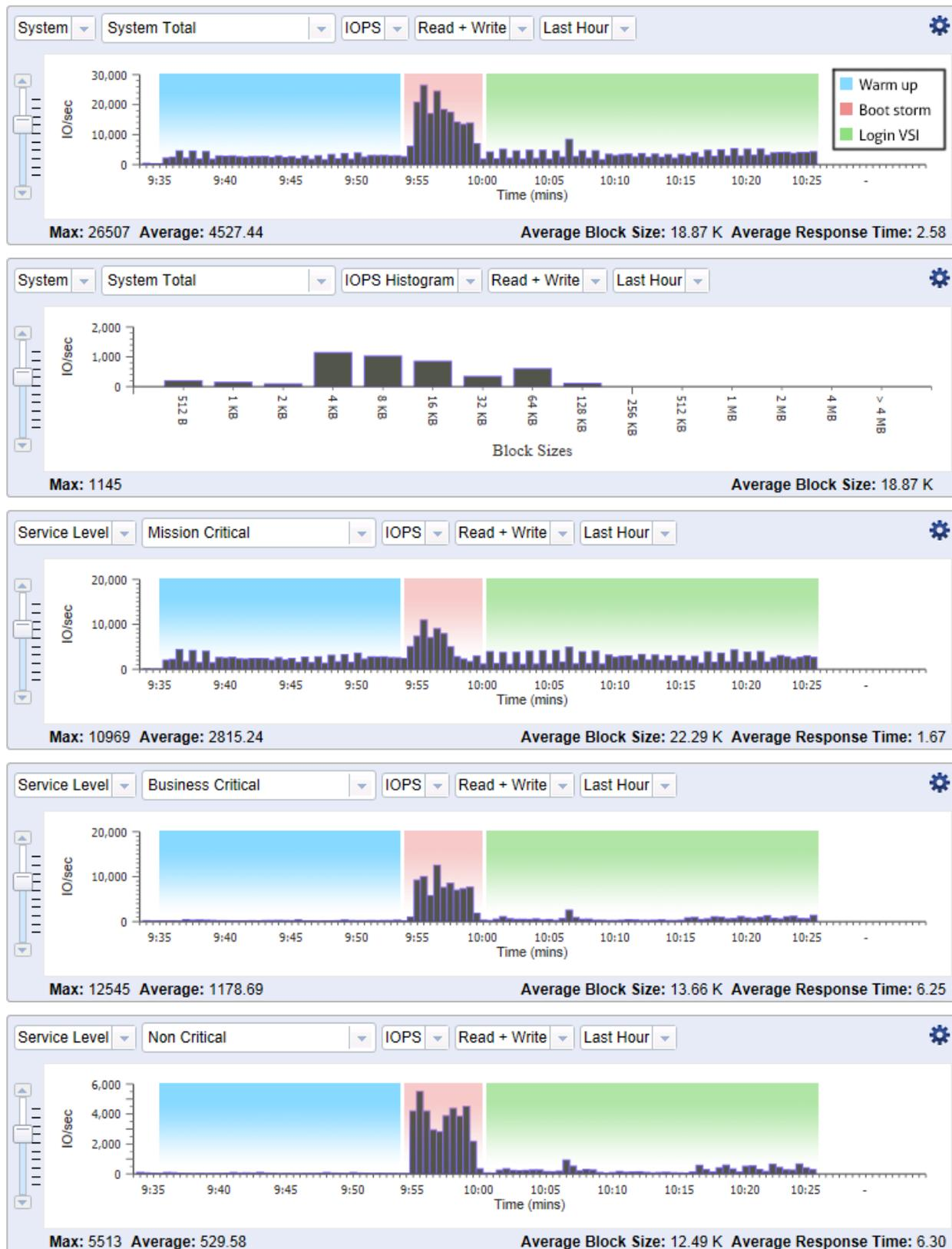
Figure 37: ioControl interface showing IOPS generated during testing.
