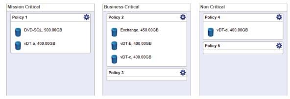
Figure 10: Configuring LUNs with the ioControl UI.
