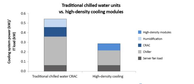
Figure 14: Traditional chilled cooling wattage versus high-density cooling module wattage.<sup>42</sup>
