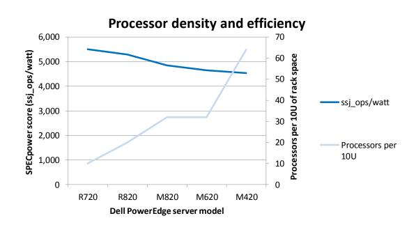
Figure 13: Dell PowerEdge servers and the relationship between processor density and power efficiency.
