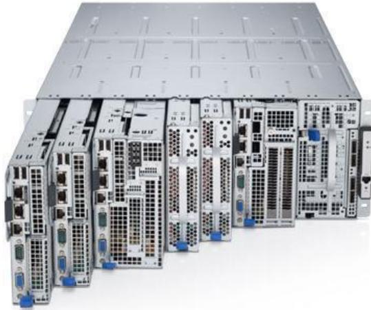
For hyperscale environments, the Dell PowerEdge C8220 microserver with the PowerEdge C8000 chassis offers very high density. The platform combines compute, GPU, and storage nodes designed to run multiple applications in a single chassis.
