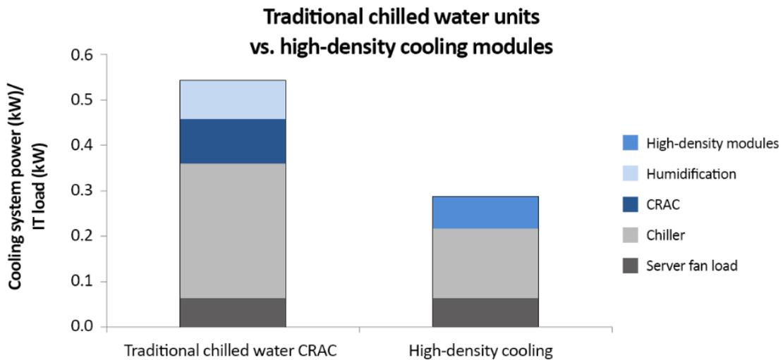
Figure 14: Traditional chilled cooling wattage versus high-density cooling module wattage.<sup>42</sup>
