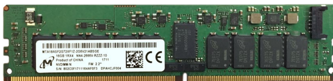
Figure 1: An NVDIMM combines NAND Flash, DRAM, and a dedicated backup power source into a single subsystem.
