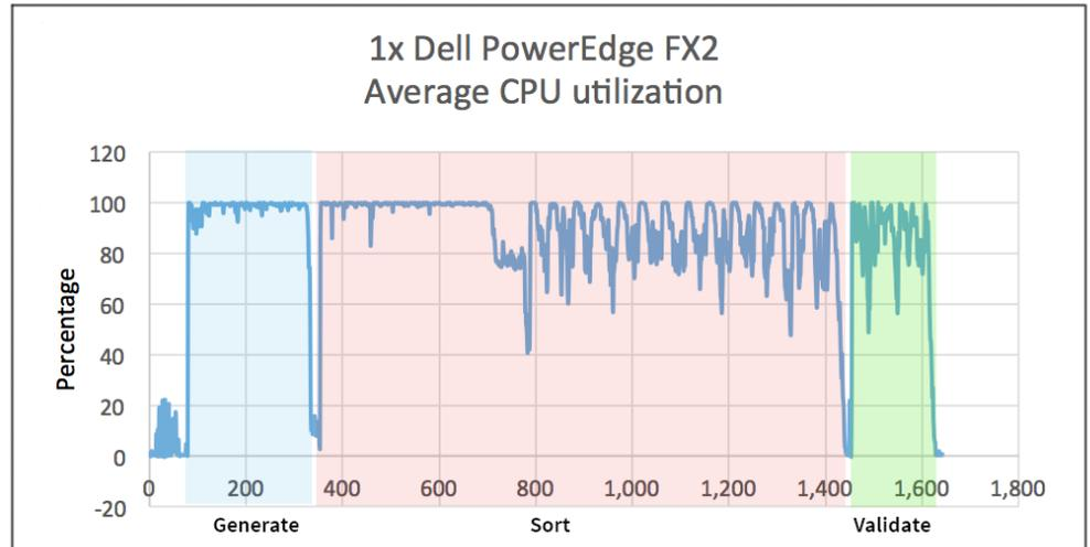
Figure 2: Average Data Node CPU utilization percentages for 1x Dell PowerEdge FX2 and for 2x Dell PowerEdge FX2.
