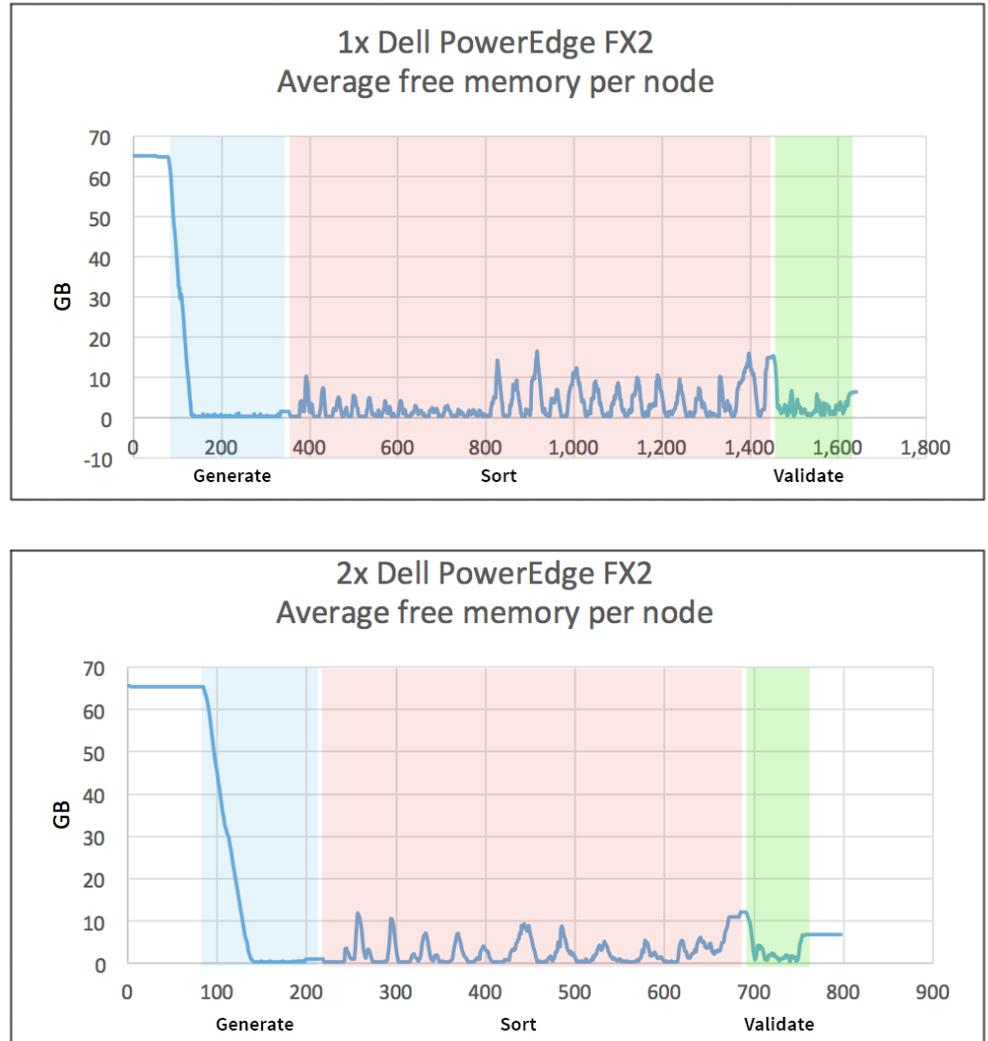
Figure 3: Average free memory per Data Node for 1x Dell PowerEdge FX2 and for 2x Dell PowerEdge FX2.
