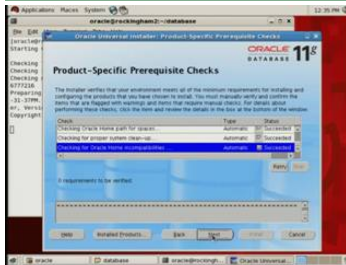
Figure 10. Checking the prerequisites.
