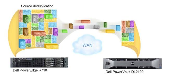
Figure 2: Source deduplication eliminates backup inefficiencies by transferring only unique chunks of data.
